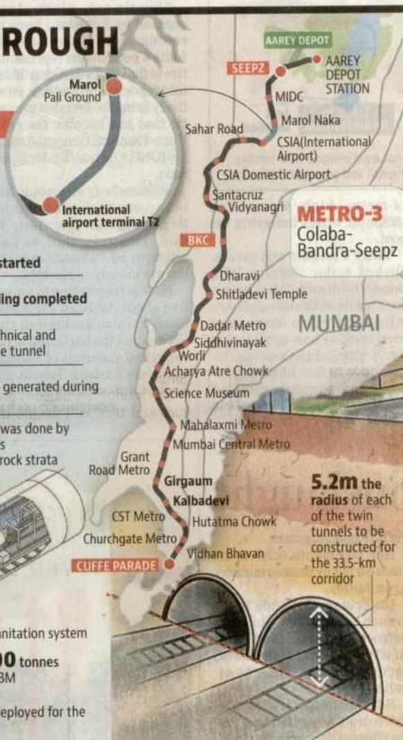
■ The first Metro-3 tunnel of 1.26km, which starts from Marol, ends at terminal 2 of CSIA. Work was completed in 259 days. SATYABRATA TRIPATHY/HT
