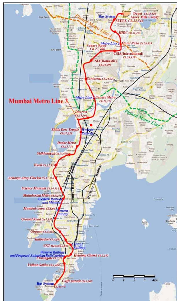
Figure 1: Alignment of Mumbai Metro Rail Line 3
